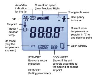
The display is handled using the buttons on the thermostat:
