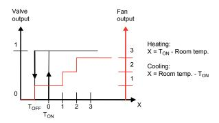
When there is no heating or cooling demand in the Auto position, the fan will run at its lowest setting. This can be changed to make the fan stop when there is no heating or cooling demand. The fan is also deactivated when in modes Off and Window. However, it will continue to run if mould protection has been configured.
