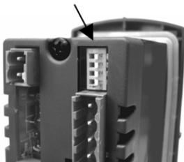
**Figure 12. DIP Switch Location**
