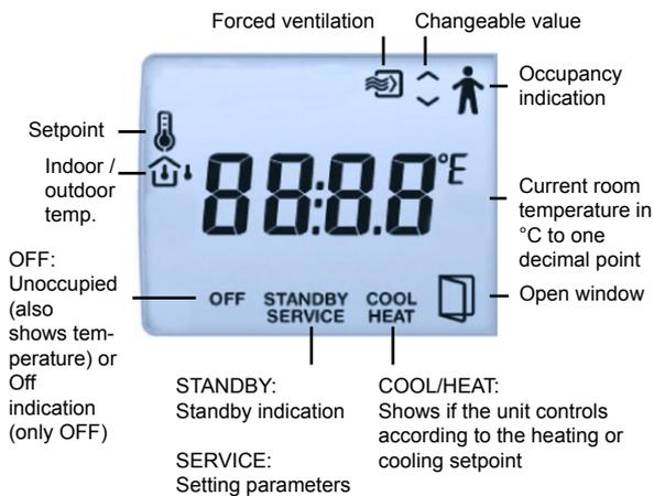
It is possible to set different parameter values in a parameter menu in the display, using the buttons on the controller. You change parameter values with the INCREASE and DECREASE buttons and confirm changes with the Occupancy button.
