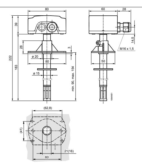
Drilling plan with (without) mounting flange
